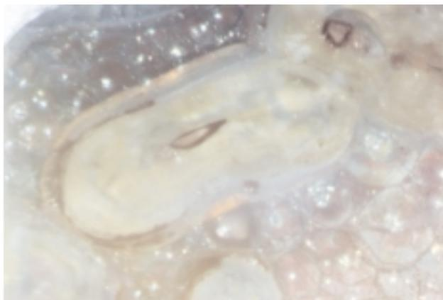
**Figure 7.** 'Ploughing' in a glass sample from Rhodes (x 3.2/0.06∞, metalographic microscope).
