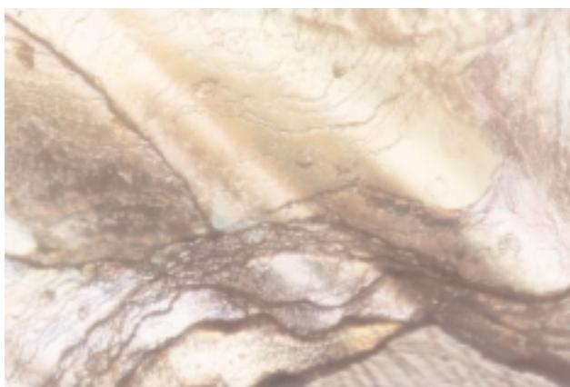
**Figure 10.** Vertical section of a groove. Layers of corroded glass that exhibit iridescence. Glass sample from Rhodes (x 10/0.20 $\infty$ , metallographic microscope).
