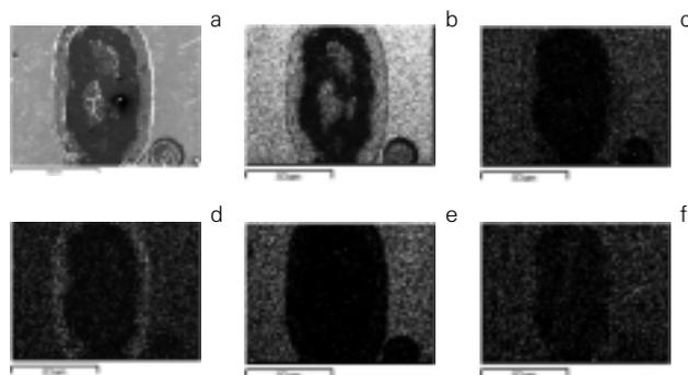
**Figure 9.** Mapping of the elements in a large pit in a glass sample from Rhodes – a) picture of the pit (x 75, S.E.M.), b) silicon, c) calcium, d) sodium, e) aluminum, f) potassium.
