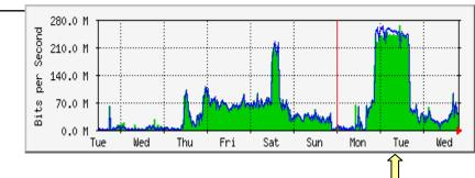
Data transfer between Spanish Tier1 and Tier2. We reached 250 Mbps using gridftp between T1 -> T2 (CCRC'08)
