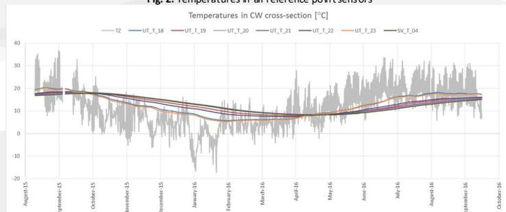
Fig. 3. Temperatures in CW cross-section
